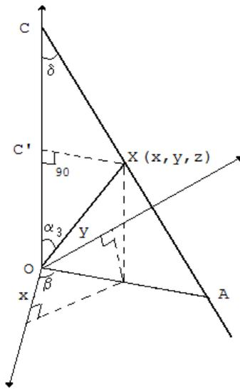
$$\overline{OX}^2 = \overline{C'X}^2 + \overline{OC'}^2 = \overline{OA}^2 (1 - \sin \mu)^2 + p^2 \sin^2 \mu$$
